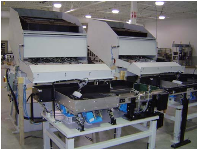
Multiple “smart dumpers” w/ flow control pans in operation. Integrated to robot assembly cell.
