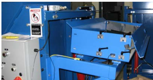
Intermediate Reduction Pan w/ Adjustable Side Guides and Flow Gate Absorbs impact load-meter parts/materials.
