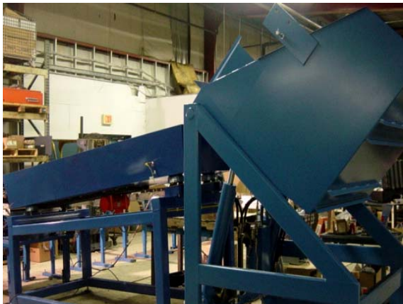
Heavy Duty Receiver Pan Feeder w/ active pan for receiving parts dumped from portable bulk containers. Pan absorbs impact load and is integrated to dumper to effectively meter parts to "on demand" upstream systems.
