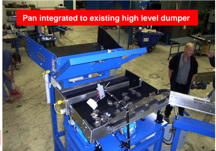
Reduction pan feeder integrated to dumper
