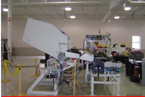
Reduction pan feeder integrated to dumper
