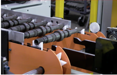
Indexing Conveyor to walking beam infeed
