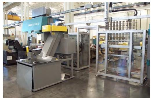
10 Cu Ft. Agitator Hopper-Machine Center
