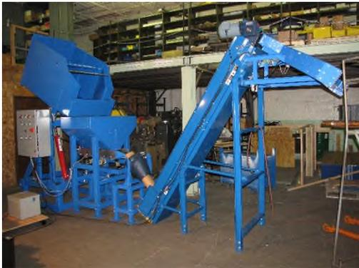
Integrated pre-feed system with automated container dumper Metering hopper, incline conveyor and splitter.- HD Faseners
