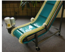
Direct Drive= Lower Horse Power & Versatile Motor Location
