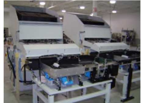
Multiple “smart dumpers” w/ distribution pans in operation within an robot assembly cell.
