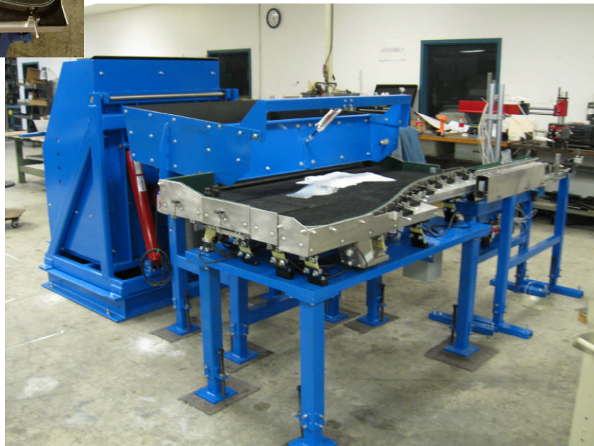
Dyna-Slide Model F4466 w/ Pan Feeder Hopper Feeds 20" bars from random bulk supply
