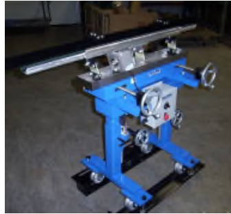
V-Track Loader with X, Z and Y Acme Adjustments
