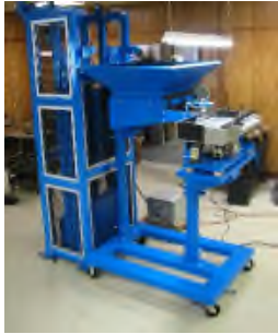
Hi Level Intelligent Tote Dunper, 5 cu ft pedestal hopper F1463 Feeder w/ custom tooling
