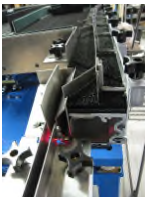
Part orientation to rolling attitude for supply to side grinder
