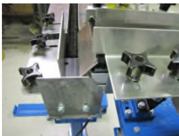
Part orientation to rolling attitude for supply to side grinder
