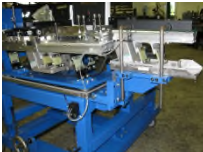
V-Track Discharge w/ Back Pressure Control & Drip Pan w/ Well Return Angle
