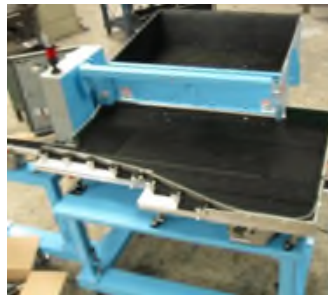
Large Part Feeders from random bulk supply
