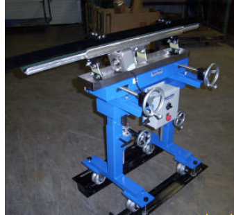
Simple Feeder- V0336 w/ x, x & z adjustment features
