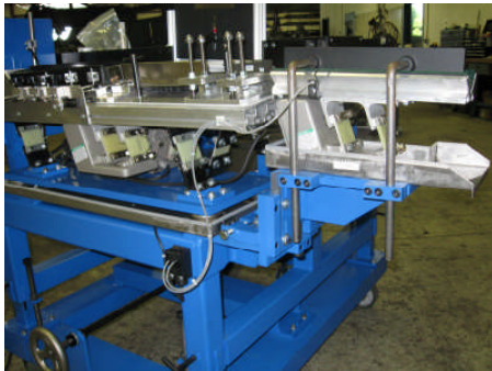
Feeder w/ Horizontal Supply Hopper X, Z adjustor, Back Pressure Control & Drip Pan w/ Well Return Angle
