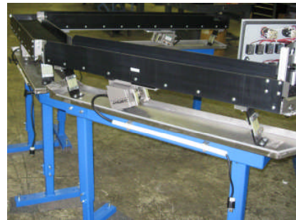
Transport & Accumulation Conveyors to operator side of grinder w/ drip pans
