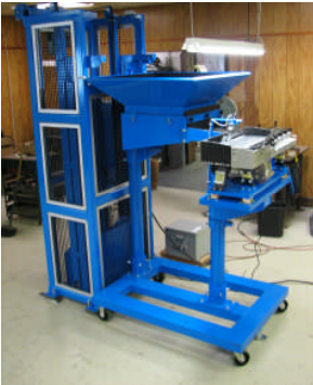
Hi Level Intelligent Tote Dunper, 5 cu ft pedestal hopper F1463 Feeder w/ custom tooling
