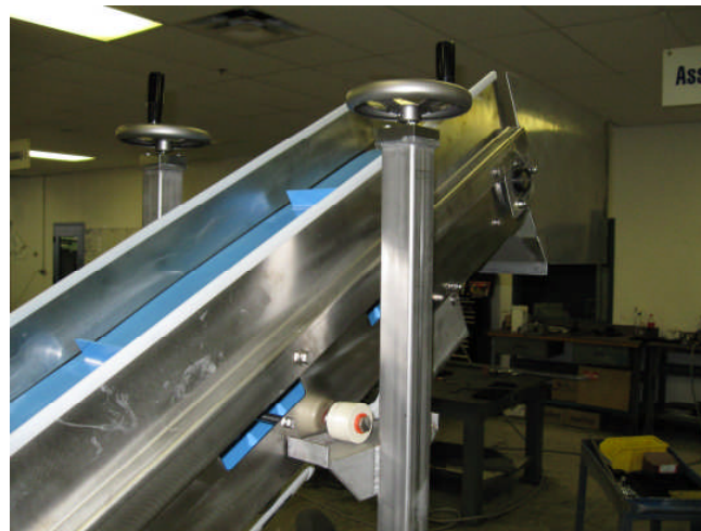
Hoppers, Height Adjustment top covers, drip pans and multiple belt options including perforated belts. Cleats and Accordion Side Aprons to 4.5" Tall
